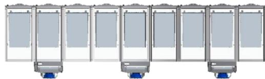
Where a room temperature of 27°C/80.6°F or below is desired (to keep with ASHRAE A1 class guidelines) USystems would assume the air off from the Cabinets without the RDC to be approximately 40°C/104°F and produce circa 600CFM. If on application this information can be provided, USystems are able to produce more accurate room temperature projections.
